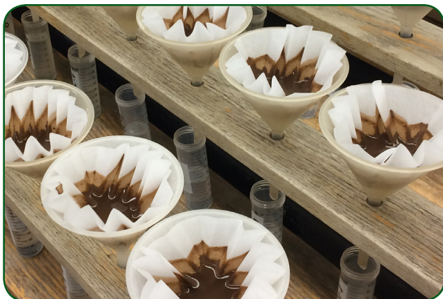
FIGURE 3. Potentially Mineralizable Nitrogen (PMN) processed in the lab. The difference between pre-incubation and post-incubation measurements of ammonium is used as an indicator of N mineralization.
