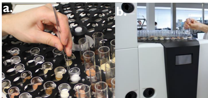
FIGURE 2. Primacs SNC-100 Carbon and Nitrogen Analyzer accepts soil or plant samples in small cuvettes placed on a carousel. Specialized software controls the insertion of each sample into the furnace, the application of combustion or purging gases, and the collection and routing of target gases to detectors for measurement.
