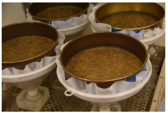
Wet Aggregate Stability Test
