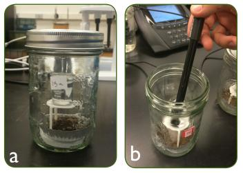
**FIGURE 3 a and b.** Soil Respiration is measured by capturing and quantifying CO<sub>2</sub> released from samples.
